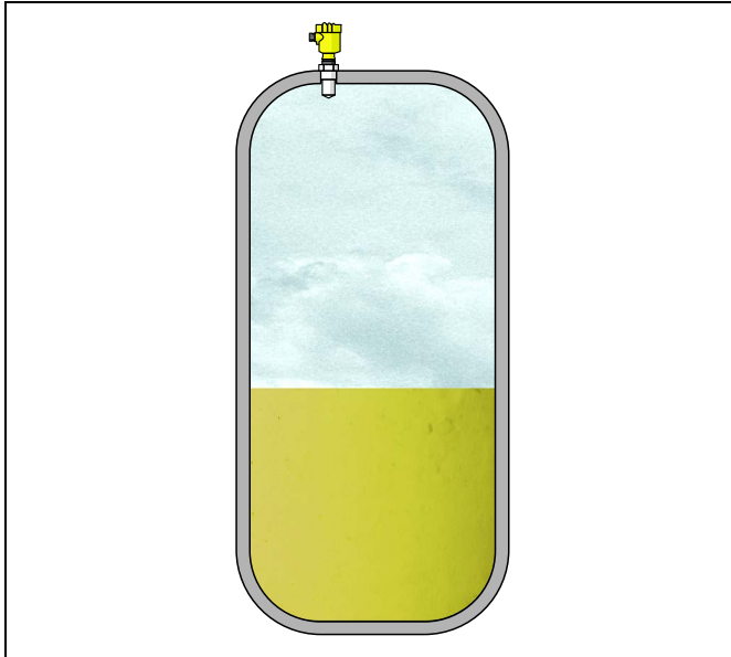
Fig. 5: Level measurement in an acid tank with VEGAPULS 61
