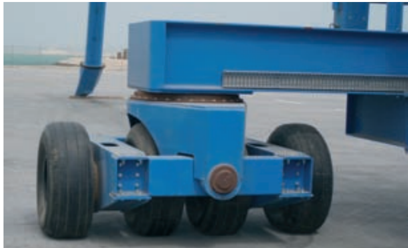
Four wheel pivoting axle assembly
