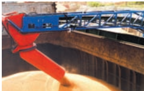
Rotating Variable Angle Chutes offer an economical solution with accurate trimming capability
