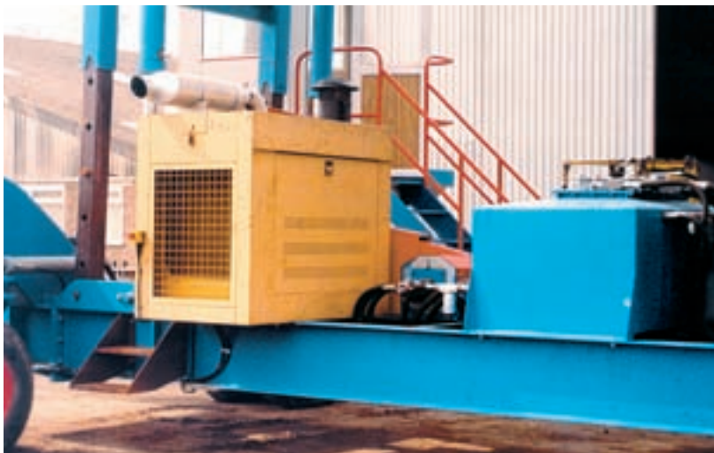
Auxiliary Gen-Set Drives the Powered Travel System Only
