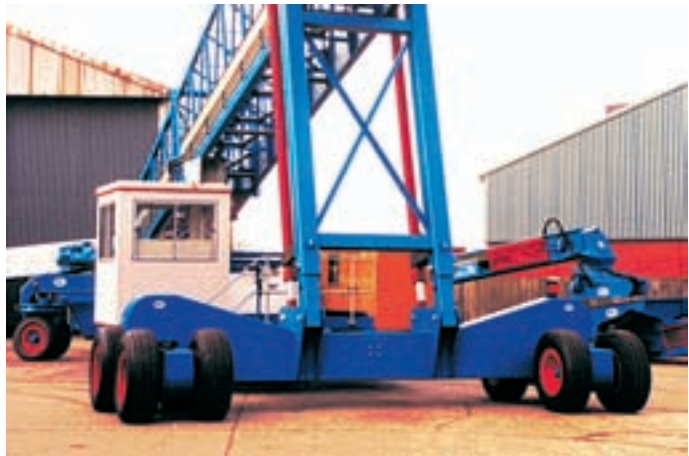
Forward Axle Beam with Telescopic Boom Supports
