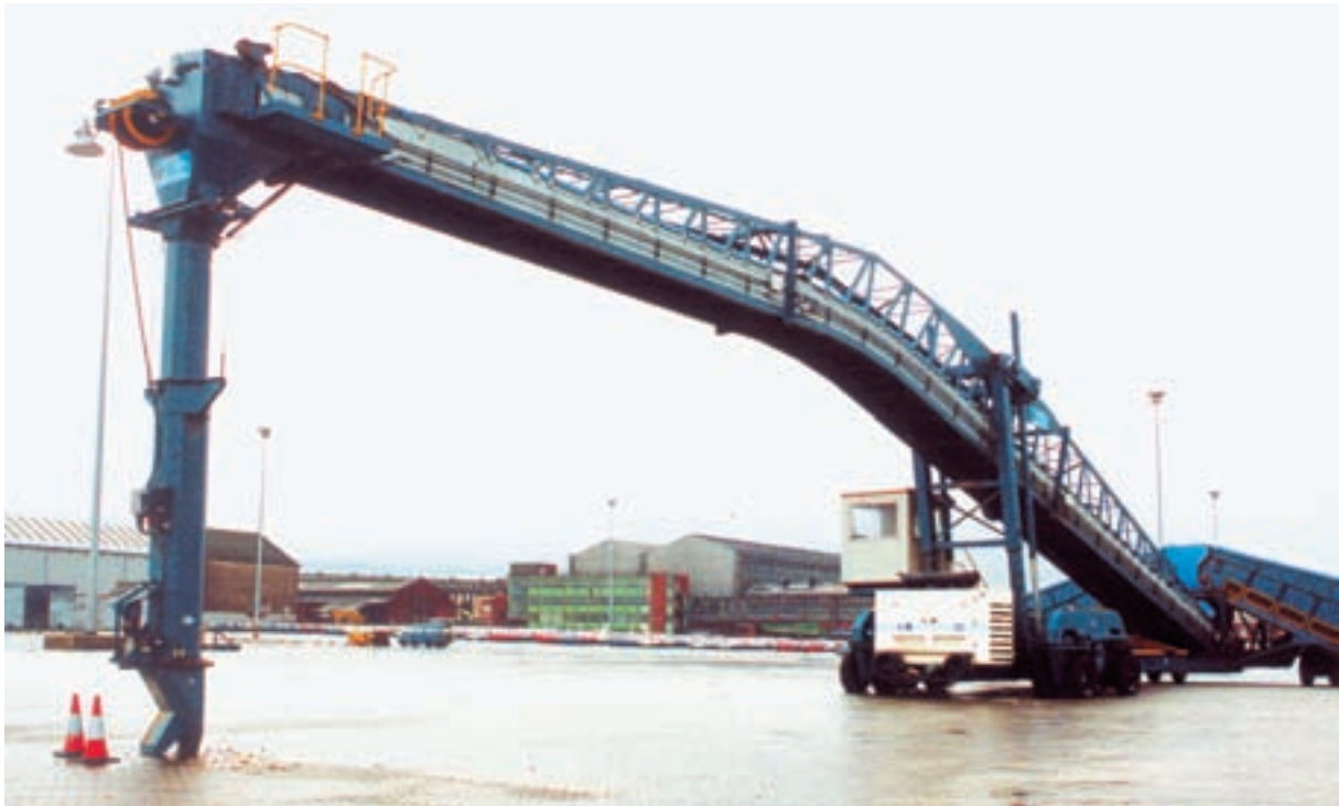
Full specification mobile Shiploader with a Variable Angle Trimming Chute and Radial Distributor
