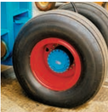
Integral Hydraulic Hub Motor
