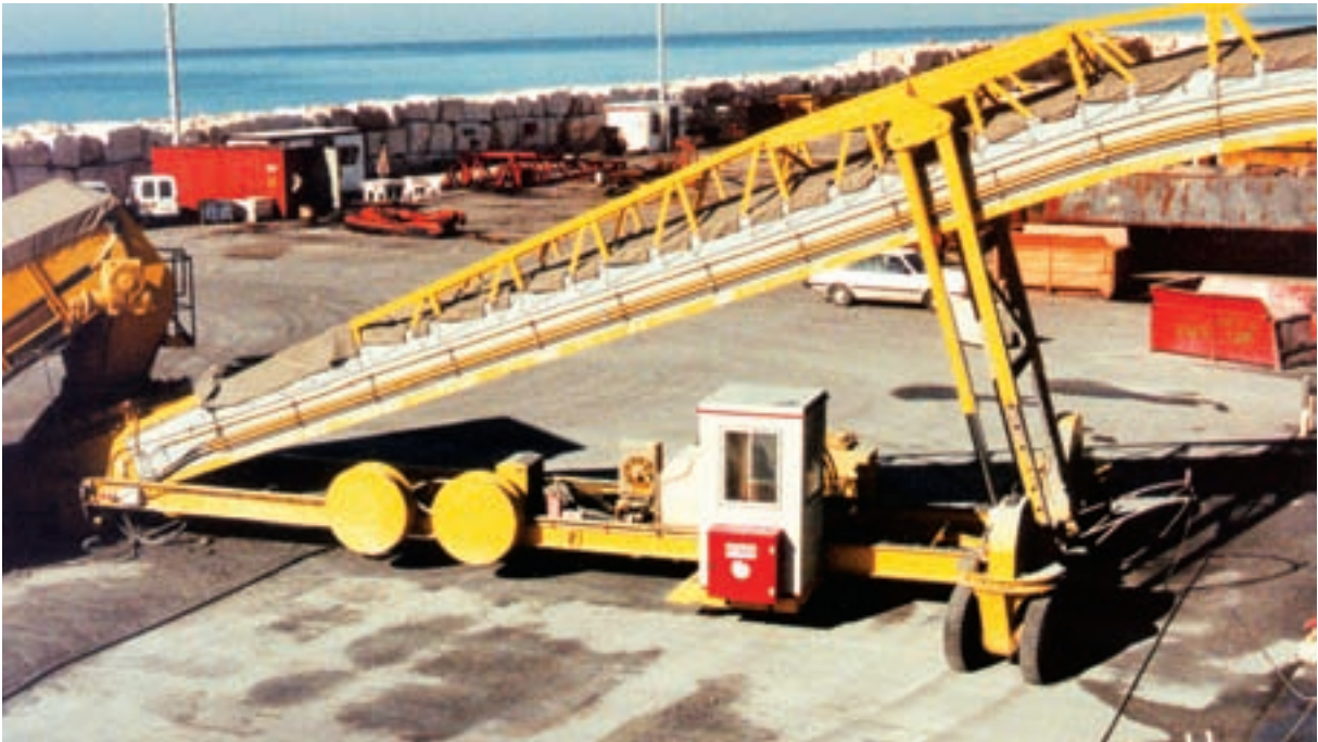
Powered Radial Operation with In-Line Tow Travel
