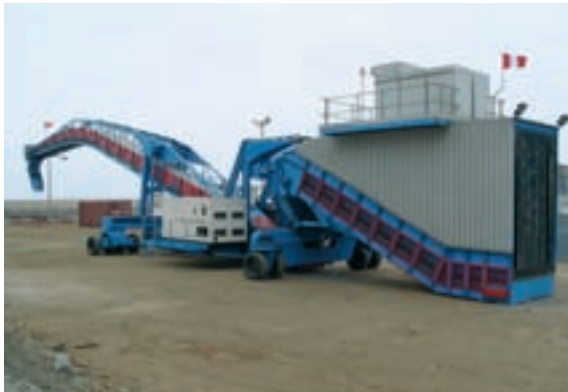
Samson™ mounted on slewing frame to Shiploader chassis.
