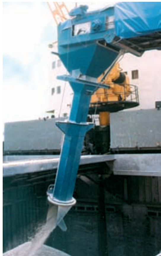
Two stage variable angle and telescopic trimming chute
