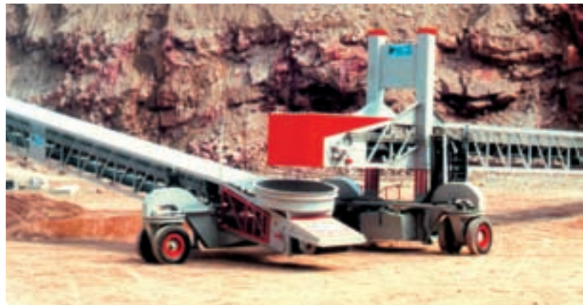
Link Conveyors with Powered Travel and Full Manoeuvring Facilities
