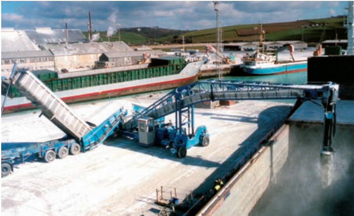
Twin integral Samson™ feeders mounted to the Shiploader chassis
