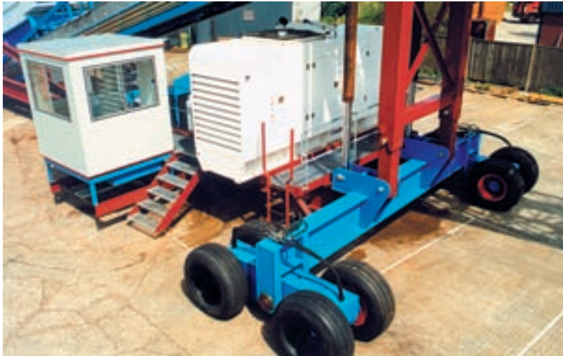
Diesel Gen-Set drives the complete Shiploader and Feeders
