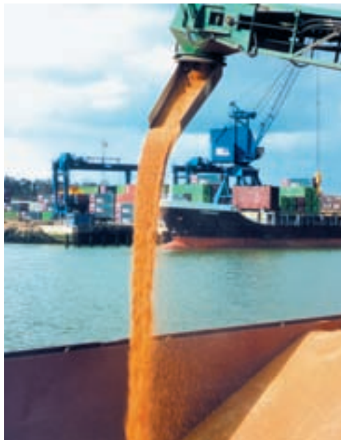
Rotating Variable Angle Chutes offer an economical solution with accurate trimming capability
