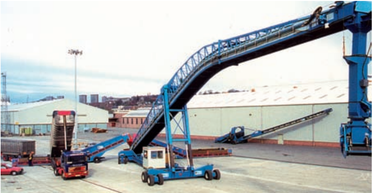
In-Line Powered Travel with Rear Steering Axles and Twin Tandem Front Axle
