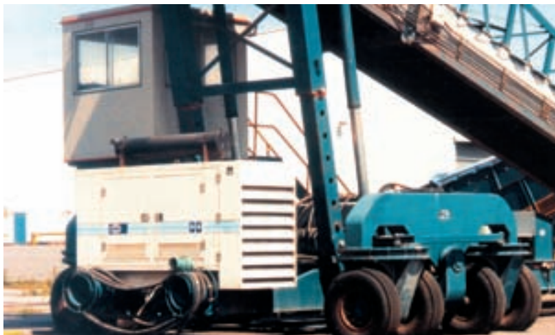
Combined Gen-Set and electric drive
