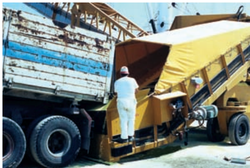
Tipping truck discharging direct to Mobile Samson™ Feeder - No Ramps Required
