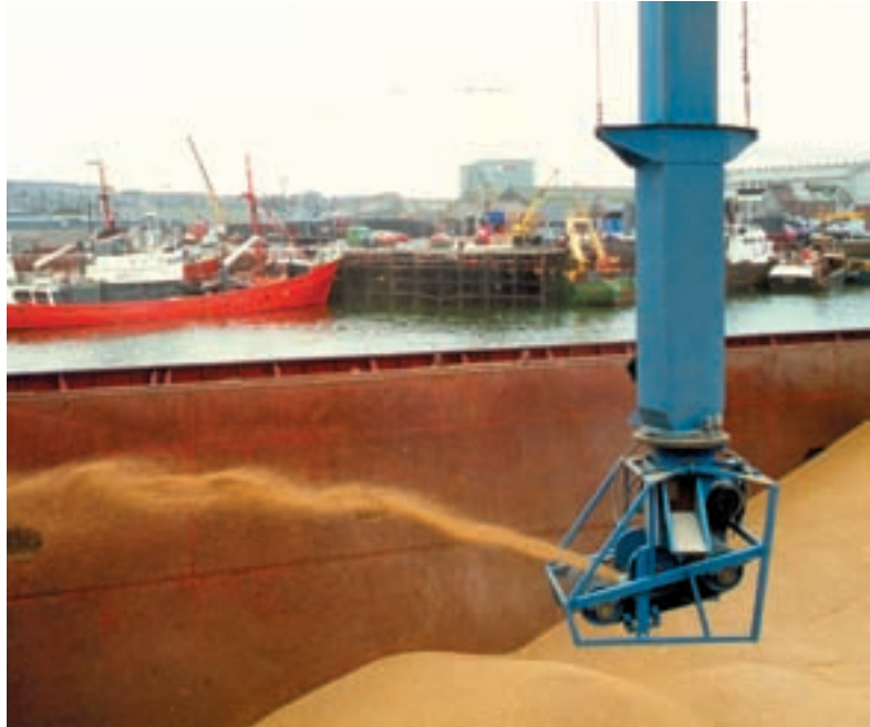
Radial Thrower provides effective trimming with minimum machine movements
