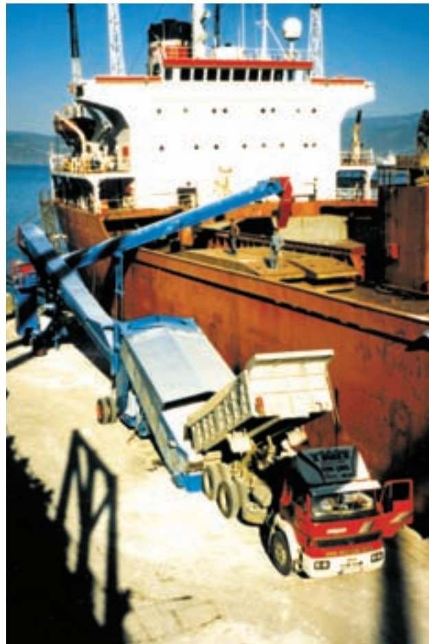
Raised chassis Shiploader with Stormajor feeder.
