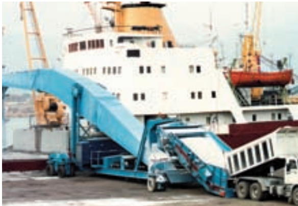
Slew Ring Mount allows the Samson™ to be positioned through 180 degree working arc
