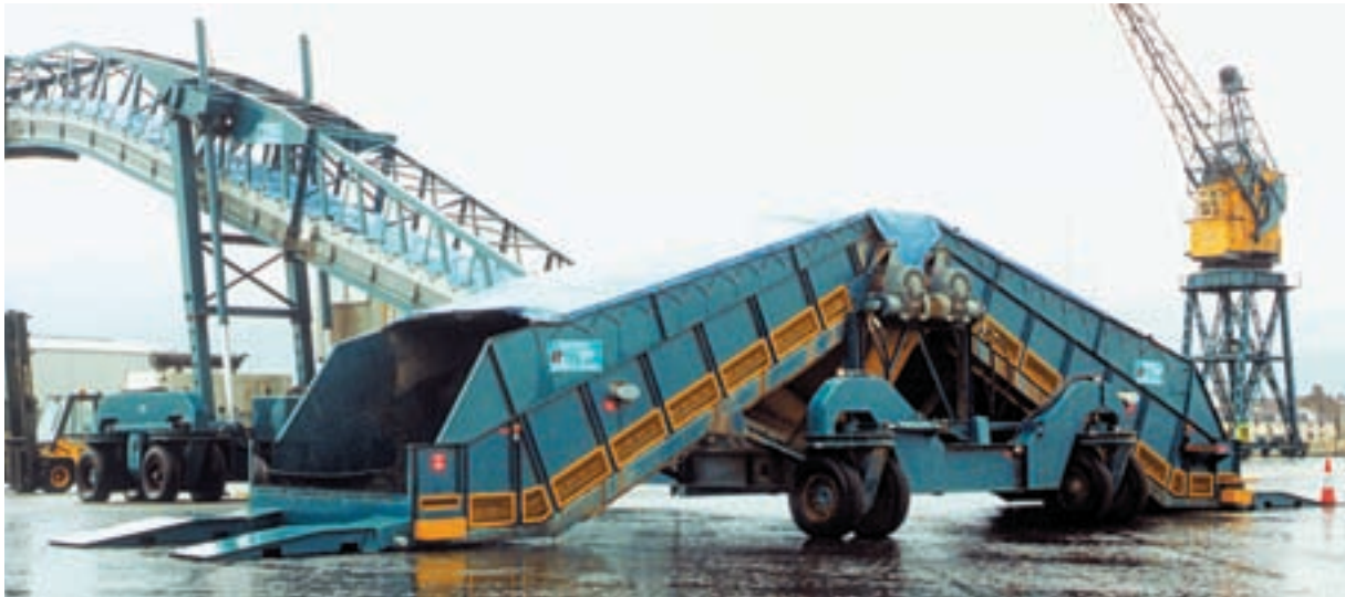
Twin Samson™ Feeders with Flexible Enclosures
