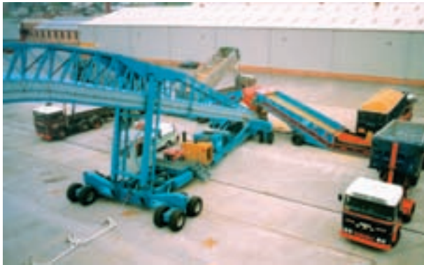
Twin independent Multi-Feed-Point Samson™ feeders discharge to a single Shiploader
