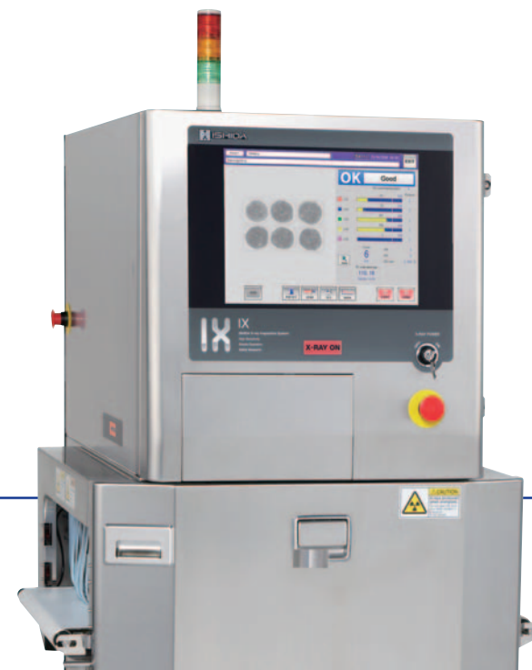
The IX-GA system is particularly effective in detecting bone fragments in, for example, chicken or pork
