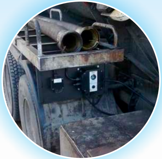
The Earth-Rite MGV static grounding system can be mounted on vacuum trucks and tank trucks.
