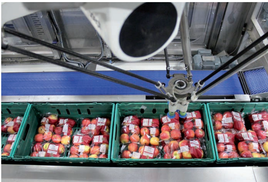
With many end-of-line packing stations now automated, incorporating vision is becoming increasingly commonplace.
