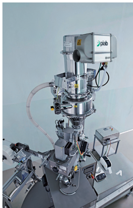
The Pi-Flow P vacuum conveyor from Piab feeds Kora's contract filling line
