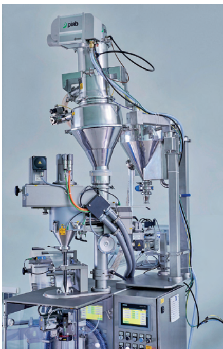
The Pi-Flow P vacuum conveyor from Piab feeds Kora's contract filling line
