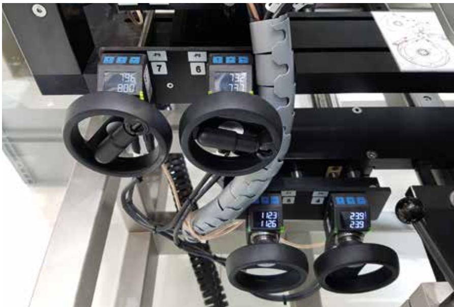
Size changeover using SIKO position indicators on a Track & Trace system in pharmaceutical manufacturing
