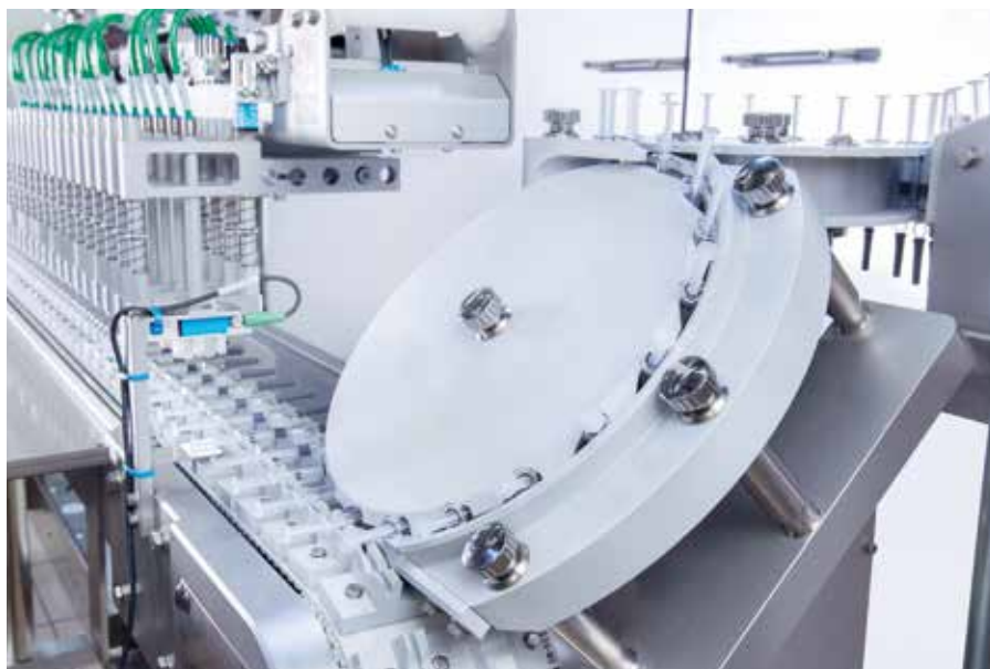
Two interlocking star wheels ensure the exact feeding of the syringes.
