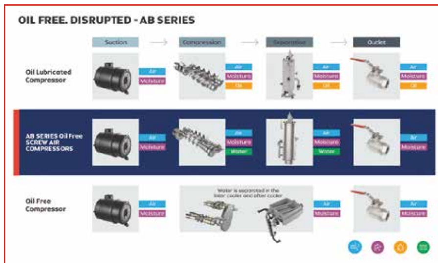
How the different components in the compressed air system assure Class 0 oil free air
