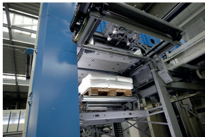
The lifting gear of the BEUMER paletpac in action. With cement, for example, the machines can achieve a throughput of up to 6,000 bags per hour. Source pictures: BEUMER Group
