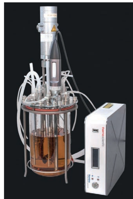
Compact sized devices allow flexible real time monitoring of biopharmaceutical processes.
