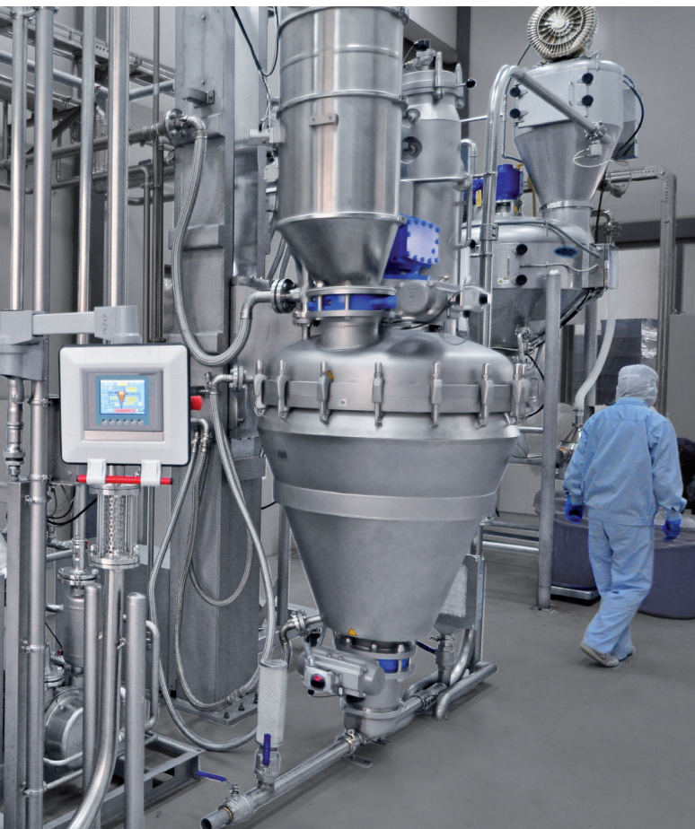
AVA supplied a special dryer suitable for handling the heat-sensitive plant proteins.
