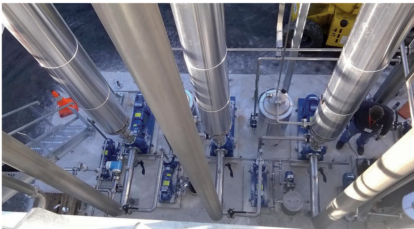
The HRS ZLD system is based on HRS Unicus Series of scraped surface heat exchangers
