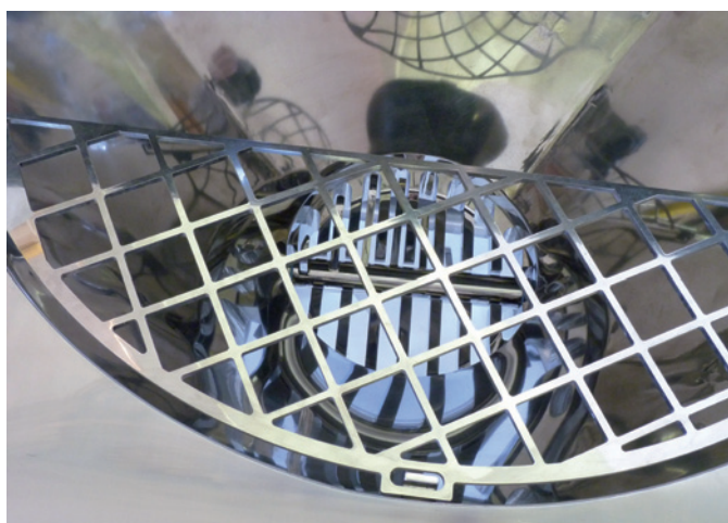
Bag breaker hopper for crushing dust. Full unit and details with HR Crusher used inside
