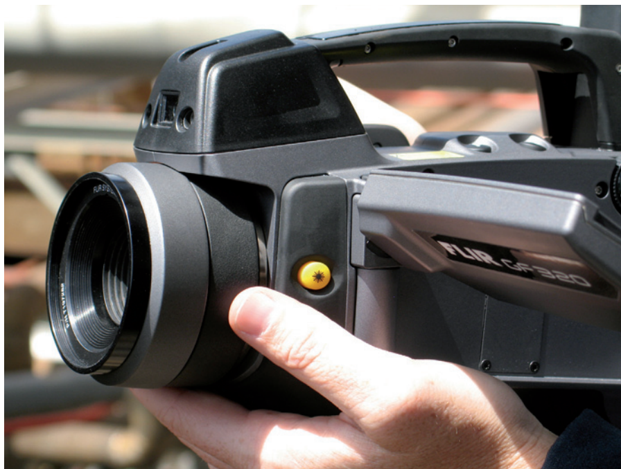
FLIR GF320 camera with a spectrally filtered indium antimonide detector and resolution of 320 by 240 pixels
