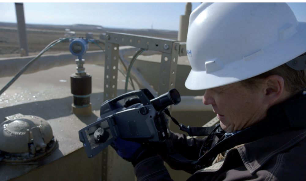
Localizing a potential gas leak at a thief hatch
