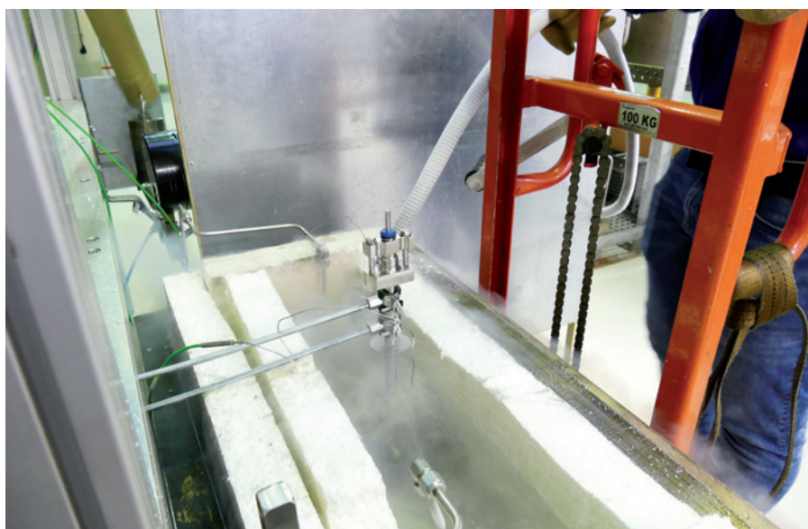
The Testing of cryogenic valves down to -196°Celsius.
