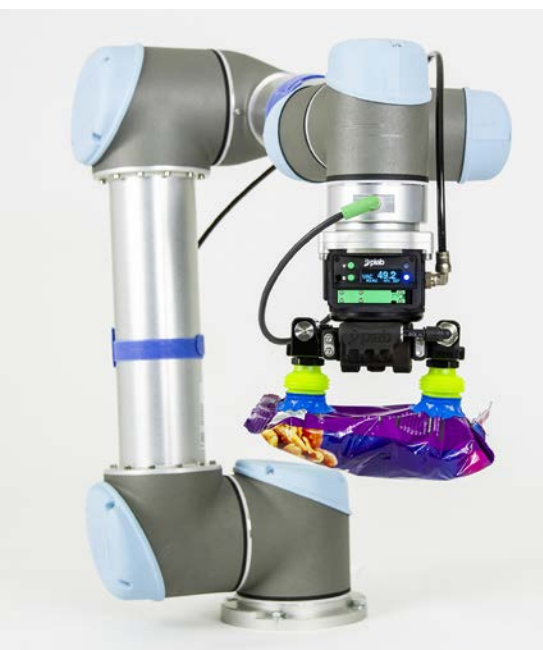
piCOBOT with piGRIP suction cups handling bags for packaging
