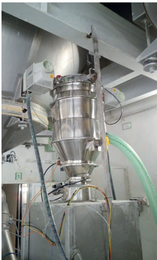
A piFLOW®p vacuum conveyor helps to assure the product quality and reduce waste.
