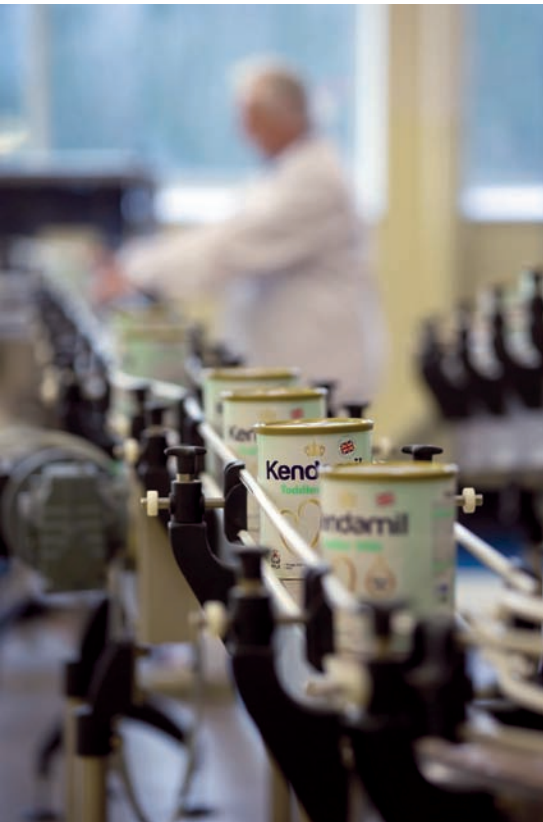
Filling lines are able to pack formulated milk in metal and composite cans, bag-in-box and sachets
