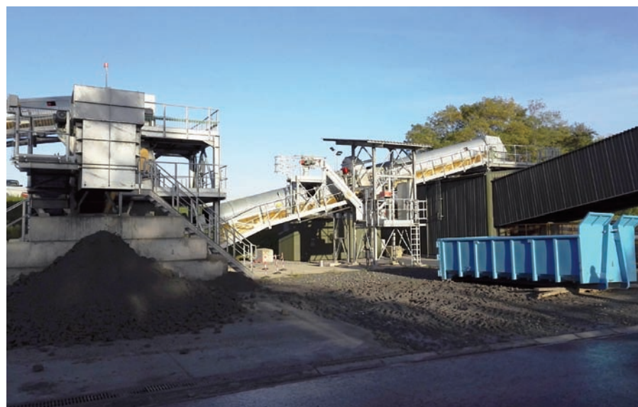
This is where the conveying begins. The material is transported from the stockpile onto the Pipe Conveyor
