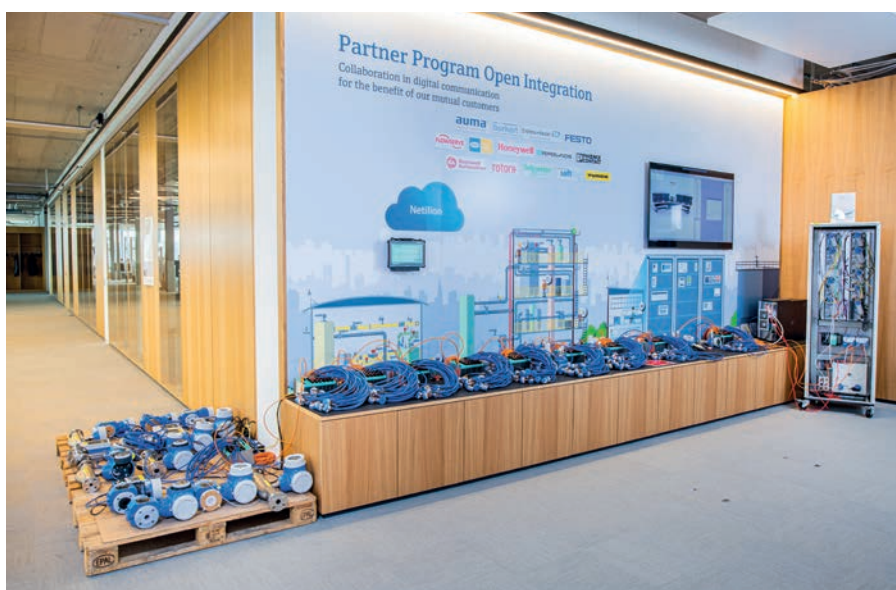
238 Endress+Hauser field devices were integrated into an Ethernet-APL system using Pepperl+Fuchs' field switches and Honeywell controls. Ethernet-APL offers a bandwidth and speed that lift field data transmission to a completely new level. Maintenance and plant managers benefit from new insights.
