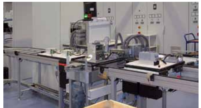
Automatic high voltage testing system
